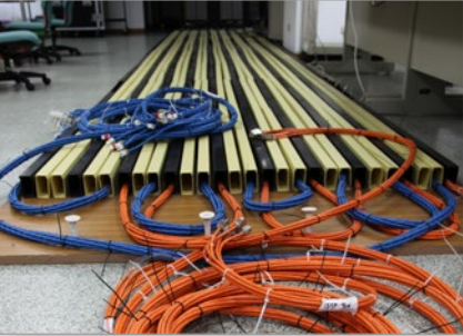
Cat 6A Channel Alien Crosstalk Test
